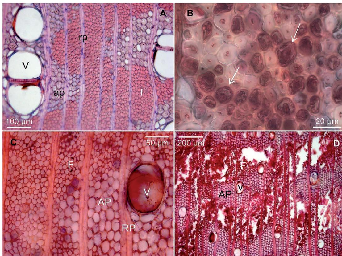
**Fig. 5.** Microscopic characterization of the sibirupura wood deteriorated by *Ganoderma australe*. A) Transverse section of sound wood. B-D) Transverse section of wood at advanced deterioration stage, with degradation of fibers cell walls, yet with intact middle lamellae and not attacked cells of the radial and axial parenchyma. Abbreviations: ap: axial parenchyma; f: fibers; rp: radial parenchyma; V: vessels.
