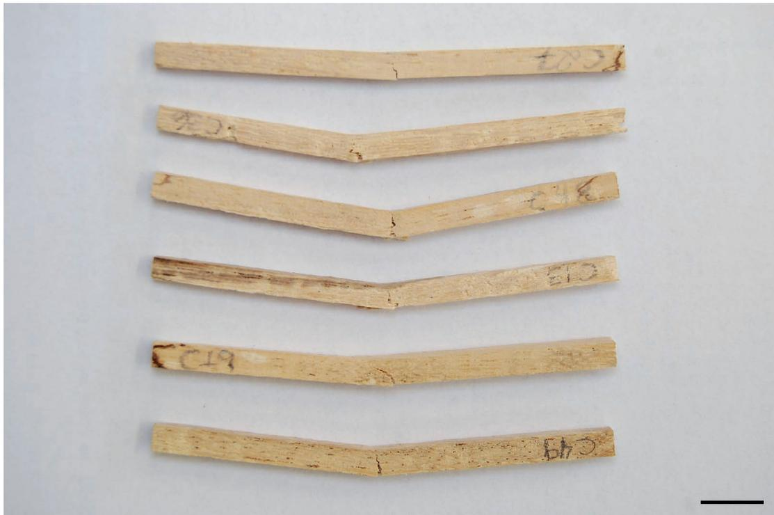
Fig. 7. Failure model in the static bending tests samples from the sibipuruna wood decayed by *Ganoderma australe*, ruptured by simple tension (scale = 1 cm).
