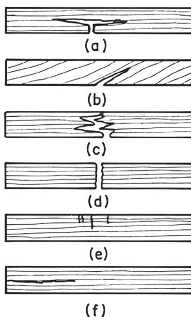
Fig. 2. Failure model in static bending. A) Simple tension. B) Cross-grain tension. C) Splitting tension. D) Abrupt tension. E) Compression. F) Horizontal shear. Source: Bodig & Jayne (1992, p. 305).
