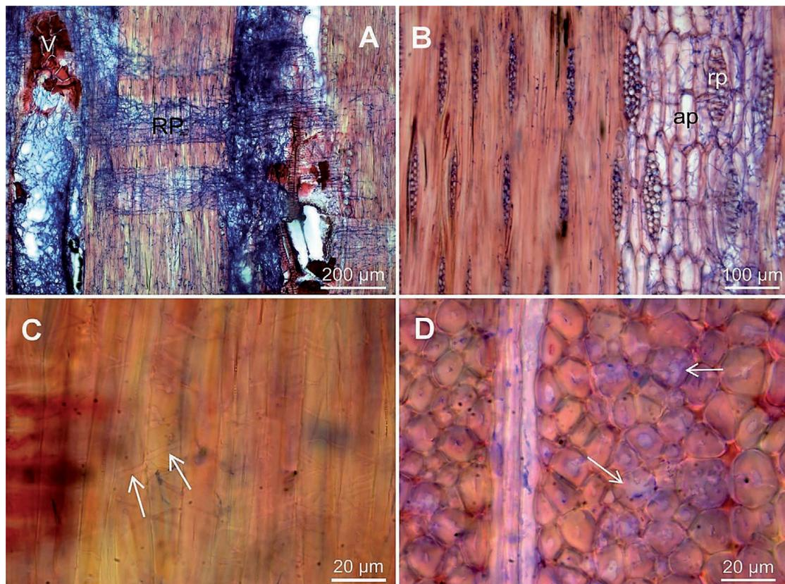
**Fig. 4.** Microscopic characterization of the sibipiruna wood deteriorated by *Ganoderma australe*. A) Radial longitudinal section. B) Tangential longitudinal section. Hyphae (in blue) intensely colonizing vessels and cells of the radial and axial parenchyma. C) Tangential longitudinal section. D) Transverse section. Erosion (arrows) of the cell wall of fibers, which is characteristic of the simultaneous white rot. Abbreviations: ap: axial parenchyma; rp: radial parenchyma; V: vessels.
