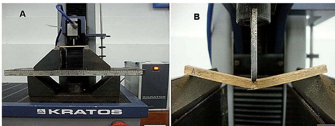
Fig. 1. A) Static bending tests on the sibipiruna wood in a universal machine. B) Specimens ruptured during the testing (scale A = 10 cm, scale B = 1 cm).
