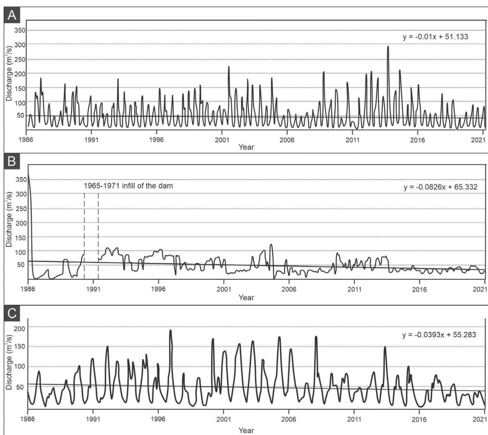
**Fig. 4.** A) Monthly discharge ( $\text{m}^3/\text{s}$ ) diminution of the Chubut River measured at Los Altares station (interval 1943-2021). B) Discharges of the Chubut River ( $\text{m}^3/\text{s}$ ) at the Ameghino Dam (interval 1961-2019). C) Monthly discharges of the Seguerr River ( $\text{m}^3/\text{s}$ ) at Los Molinos station (1986-2021 interval).
