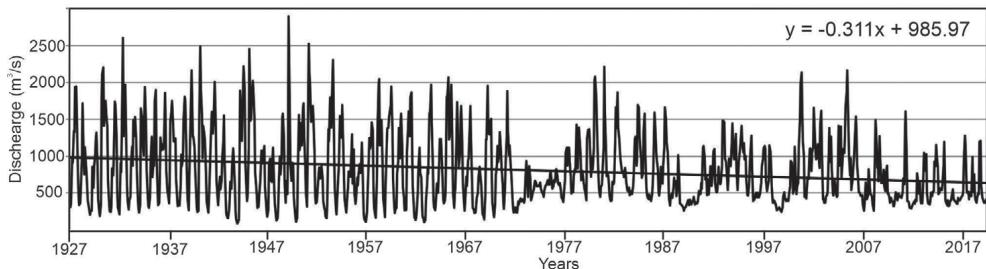
**Fig. 3.** Discharge ( $\text{m}^3/\text{s}$ ) of the Negro River at Primera Angostura (1927-2021). Floods were reduced since the dams' constructions during the seventies.
