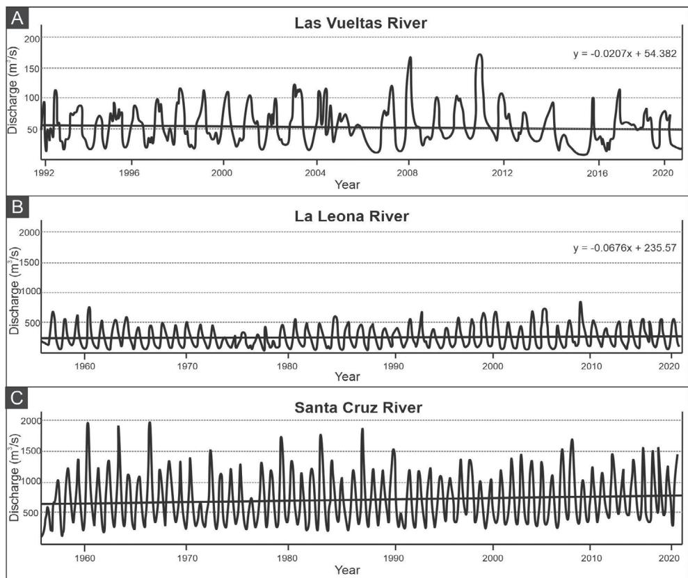
**Fig. 8. A)** Las Vueltas River station (interval 1991-2020). **B)** La Leona (interval 1956-2020). **C)** Santa Cruz River discharges ( $\text{m}^3/\text{s}$ ) at Charles Fuhr gauge station (interval 1955-2020).
